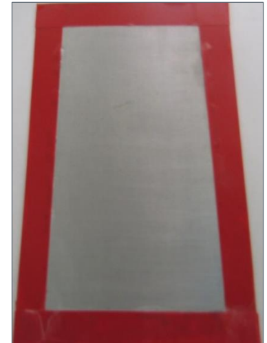
2024 alloy Picture after SST 168h
